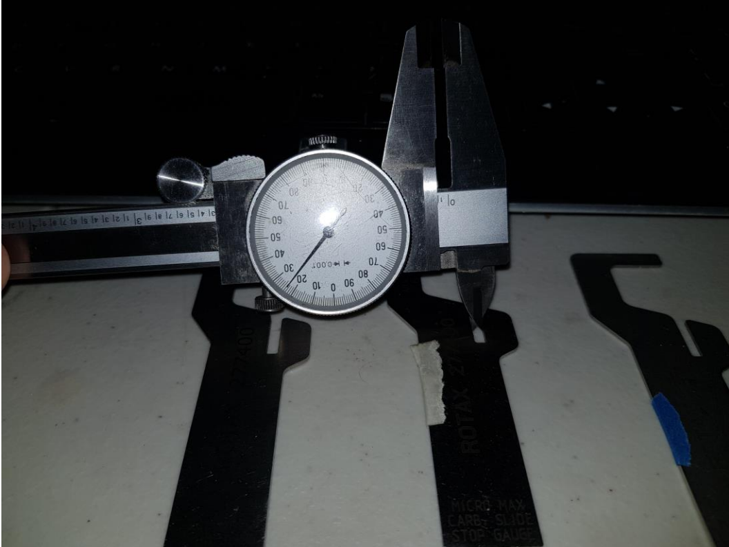
Member B tool (marked with white tape) measured float level allowance gap.
