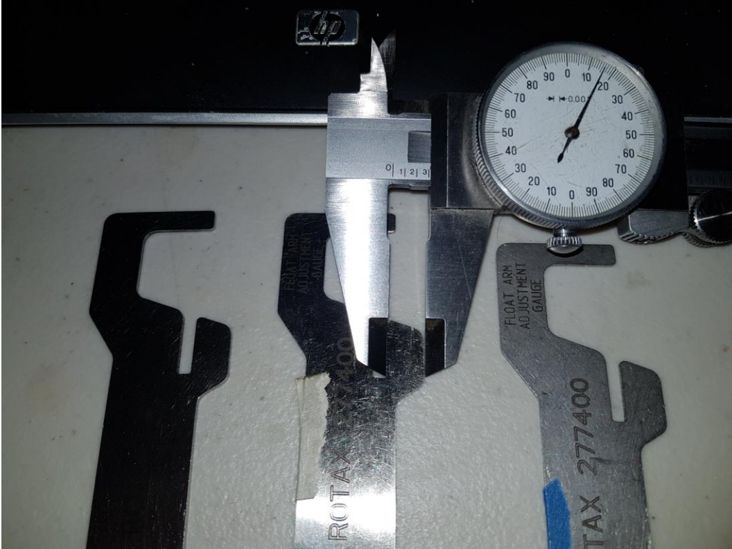
Member B tool (marked with white tape) measured for lower float level.
