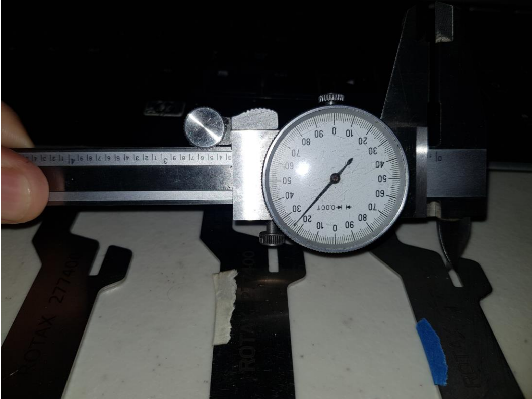
Member A tool (marked with blue tape) measured float level allowance gap.
