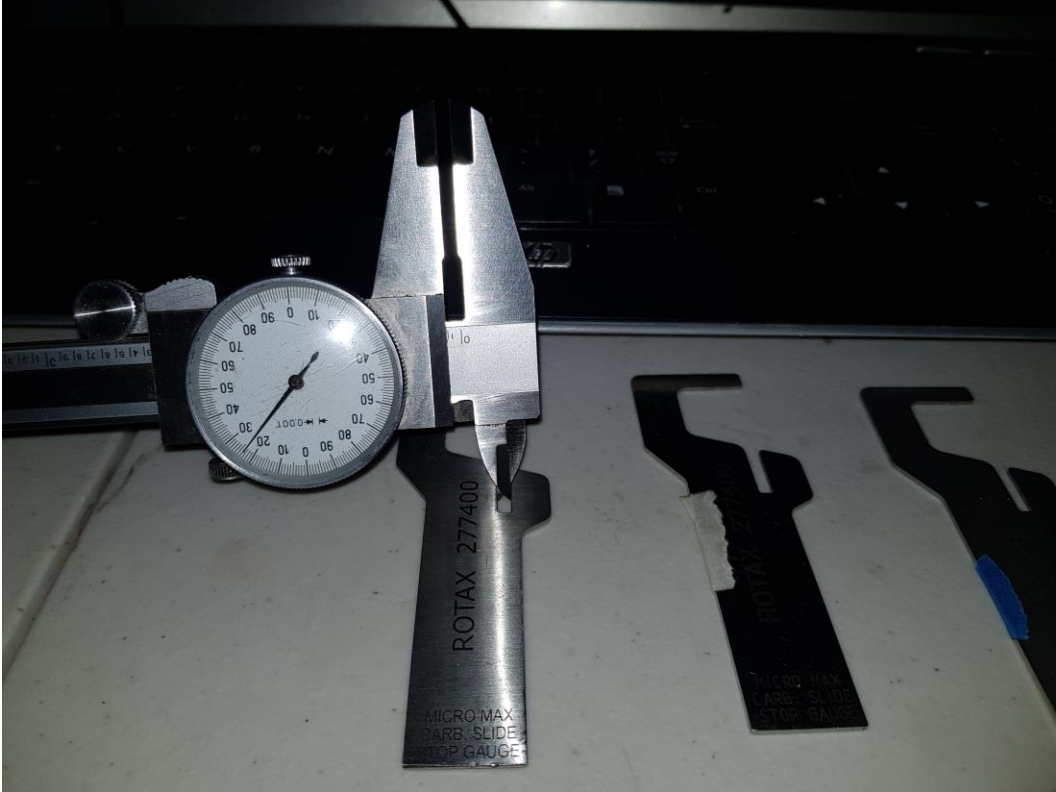
JKA tool (unmarked) measured float level allowance gap.
