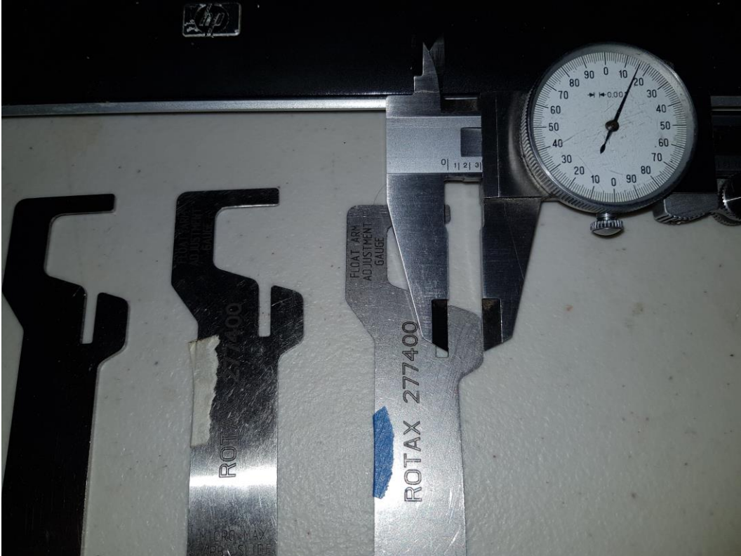
Member A tool (marked with blue tape) measured for lower float level.
